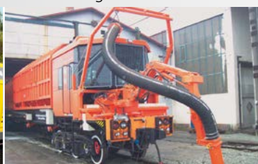
Railway vehicle for track cleaning
