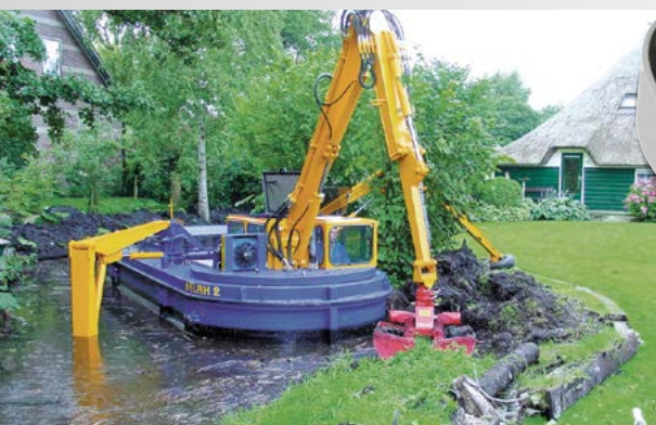
This working boat uses a WD-L slew drive for the excavator arm
