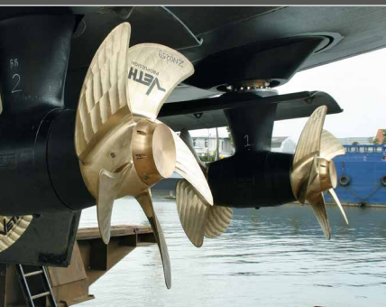
Counter rotating z-drive thruster
