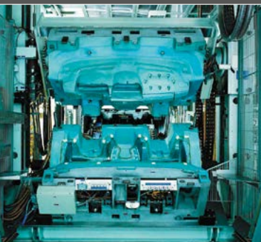
IMO slew drive for the demolding of car seats
