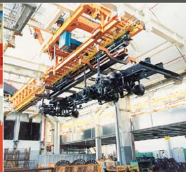
IMO slewing ring Ø 2,5 m for truck frame swivel spreader
