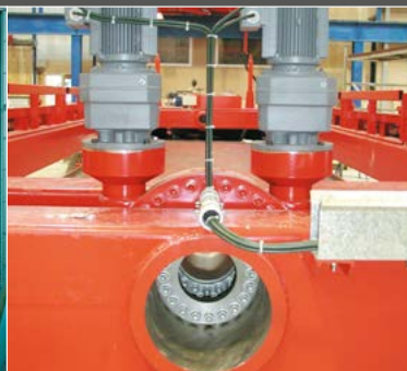
IMO slew drive turn-over device for concrete factory
