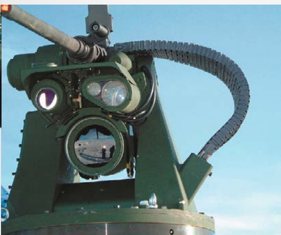
This gun turret with targeting optics is rotated by a ball slewing ring with special raceway geometry
