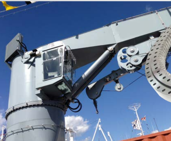
◀ Single-row ball slewing ring with internal gear for turning the loading crane on a supplier ship
