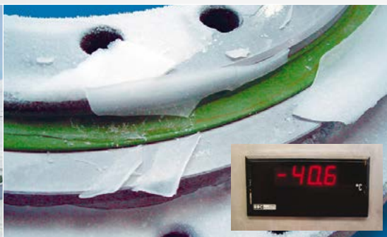
IMO slewing ring in a gun turret bearing in an environmental test above the Arctic Circle under extreme weather conditions
