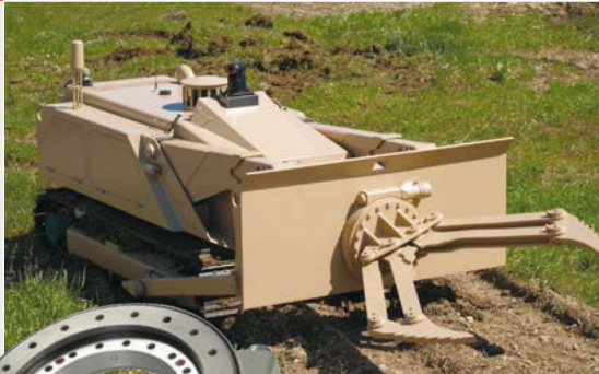
Mine clearing device with a WD-L series slew drive
