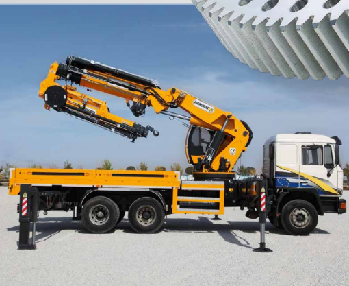
A double row ball slewing ring is used in this loading crane
